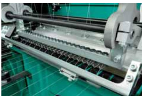
Weft laying system Schusslegesystem
