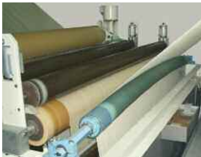
Banana roller Bananenwalze
