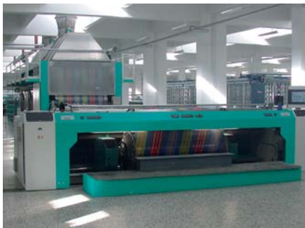
Fig. 7: Overhead cylinder dryer
