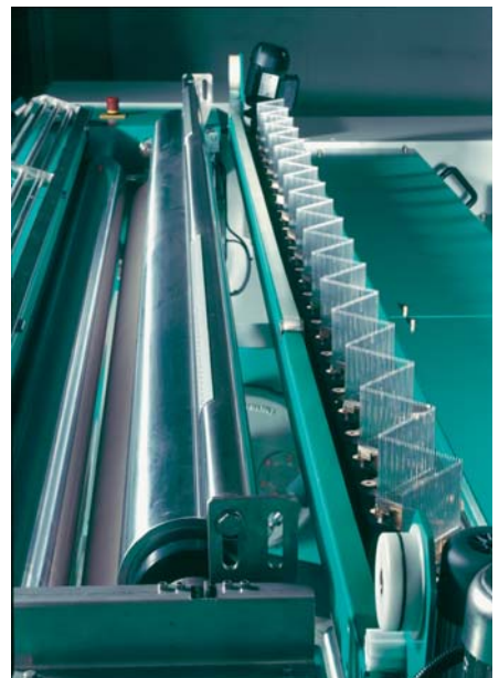
Fig. 9: Drawing-in roller and main drive of the beaming machine
