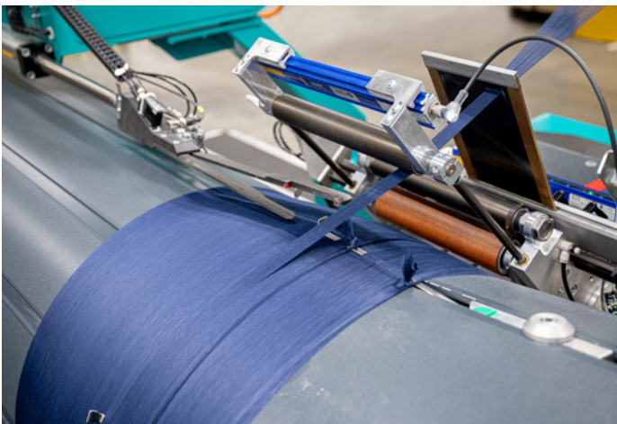
Warping table with automatic pulling rod system and duo rollers with an automatic opening and evener roller
