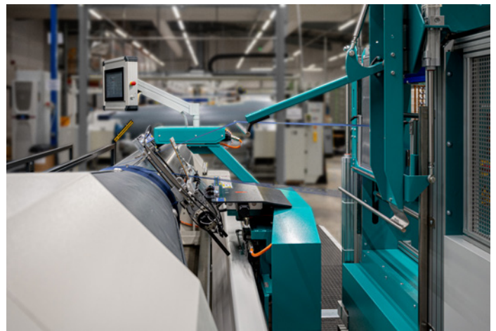
Automatic shed opening with shed separation support and laser-shed-monitoring
